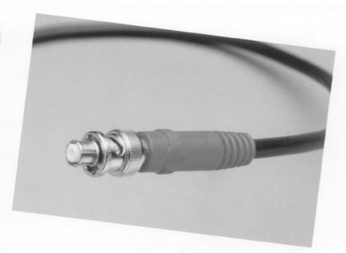
The 21 Series assembly features a molded-on strain relief that enhances the internal mechanical termination of the SHV connector to RG-59 coax cable. This provides a clean, ergonomically pleasing, cost efficient assembly.
